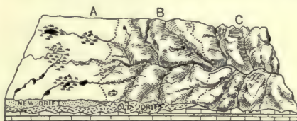
FIG. 217.—Diagram to illustrate the topography and drainage on new drift (A), old drift (B), and an unglaciated area (C).
